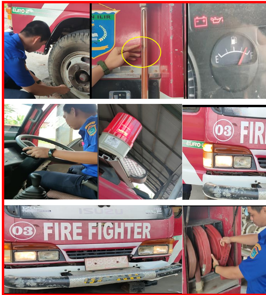
Gambar 3.7 Pelaksanaan Pengecekan (Preventive Maintenance)
